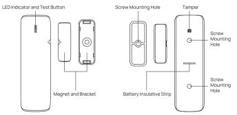
\* Corresponding the triangle of the magnetic stripe to the transmitter's to get the best detection effect.
